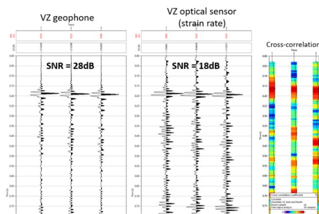
**Figure 5** Left: VZ geophone at three common depths around 1000m MD with optical sensors VZ component (middle) and correlation factor on the right (red is correlation 1 around first arrival at 180ms). SNR from optical sensor is worse than geophone but shows good character match.
