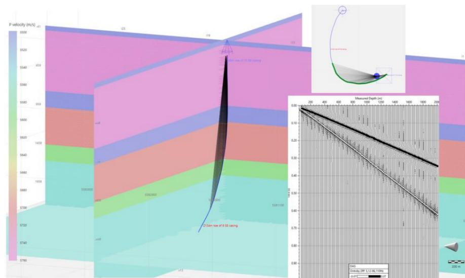
**Figure 1** Zero offset VSP geometry. 3D view and map view of direct P-arrivals. Bottom right show 2.5D ray traced filtered synthetic direct P and P&S arrivals on vertical component only (DAS amplitudes).
