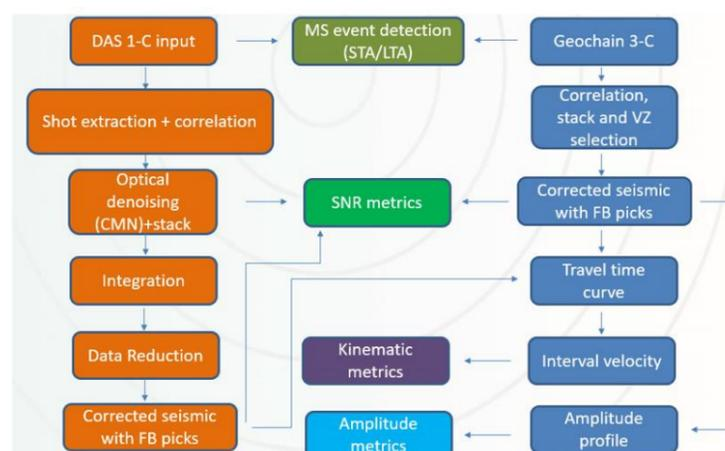
**Figure 2** DAS and 3-C wireline sensors data analysis workflow. The 3-C sensor data is the reference to generate true reference for the quantitative evaluation and comparisons of the DAS VSP data quality.
