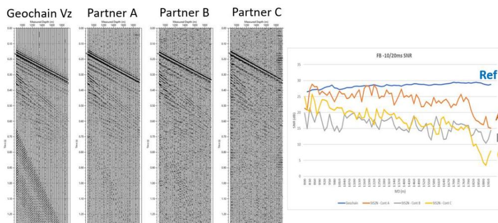
**Figure 4** Left: VZ geophone stacked reference versus DAS for partners A, B and C after pre-processing. Right: First break P-wave SNRs on VZ geophone reference and pre-processed DAS data from the three different DAS partners.
