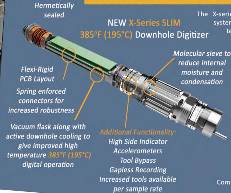
The X-series digitizer upgrade for the Geochain system, provides higher operating temperatures and higher telemetry rates, allowing continuous monitoring in the most hostile well conditions.
